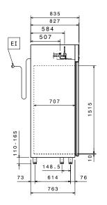
El = Electrical inlet (power) RI = Refrigerant Inlet RO = Refrigerant Outlet
